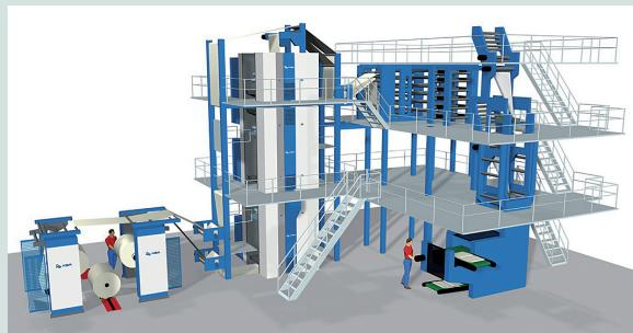
The KBA Colora at Independent Newspapers in Dover, Delaware, U.S.A., is designed for variable formats. It combines the productivity of a 4/2 press with the flexibility of a single-width press. The two folder formers are set at a 90° angle to the direction of web travel.
