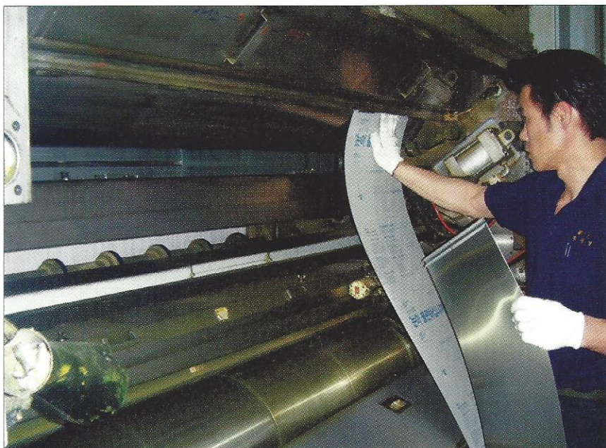
Full-circumference plates are nothing new in some newspaper markets. Here, an operator in a South Korean plant prepares to mount a doublewide press with double-long Fuji plates.
